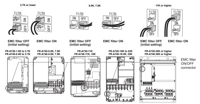
The FR-A720-0.4K and 0.75K are not provided with the EMC filter ON/OFF connector. (The EMC filter is always valid.) **<How to disconnect the connector>**
