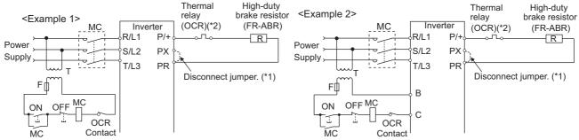
Since the 11K or higher inverter is not provided with the PX terminal, a jumper is not need to be removed. \*1
