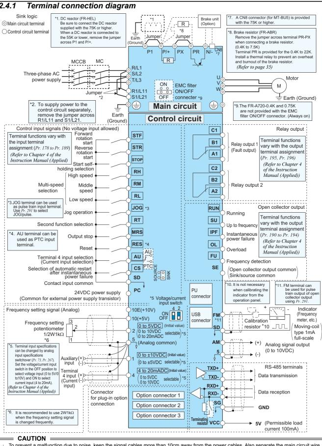
To prevent a malfunction due to noise, keep the signal cables more than 10cm away from the power cables. Also separate the main circuit wire of the input side and the output side.
