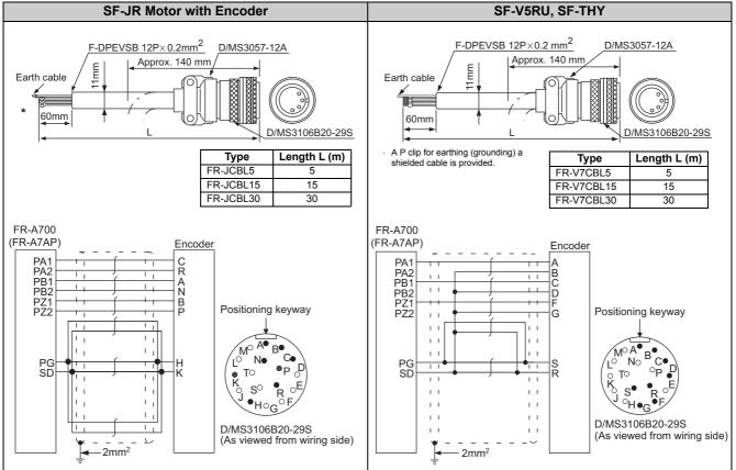
As the terminal block of the FR-A7AP is an insertion type, earth cables need to be modified. (See below)
