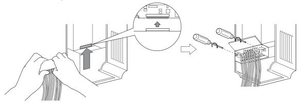
Before starting inverter replacement, switch power OFF, wait for at least 10 minutes, and then check the voltage with a tester and such to ensure safety.
