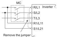
When a fault occurs, opening of the electromagnetic contactor (MC) on the inverter power supply side results in power loss in the control circuit, disabling the fault output signal retention. Terminals R1/L11 and S1/L21 are provided to hold a fault signal. In this case, connect the power supply terminals R1/L11 and S1/L21 of the control circuit to the input side of the MC. Do not connect the power cable to incorrect terminals. Doing so may damage the inverter.
