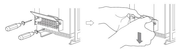
2) Change the jumper connector set to the sink logic (SINK) on the rear panel of the control circuit terminal block to source logic (SOURCE).
