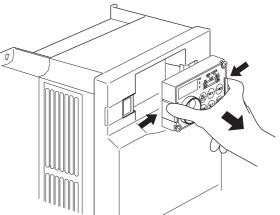
When reinstalling the operation panel, insert it straight to reinstall securely and tighten the fixed screws of the operation panel. (Tightening torque: 0.40N·m to 0.45N·m)
