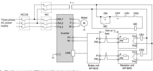
\*1 When the power supply is 400V class, install a stepdown transformer.
