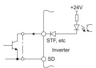
External signal input using transistor
