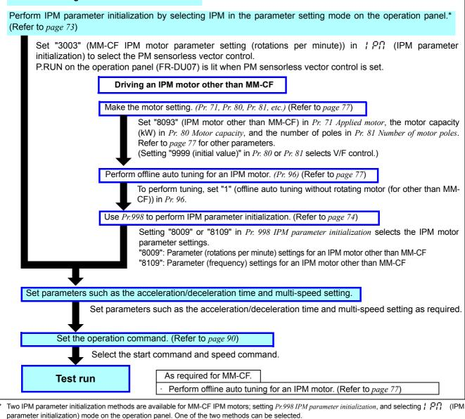
To change to the PM sensorless vector control, perform IPM parameter initialization at first. If parameter initialization is performed after setting other parameters, some of those parameters will be initialized too. (Refer to *page 75* for the parameters that are initialized.)
