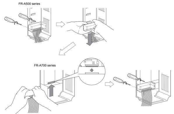
(Note that the relay output 2 (A2, B2, C2) specific for the FR-A700 series cannot be used with the FR-A500 series terminals.)
