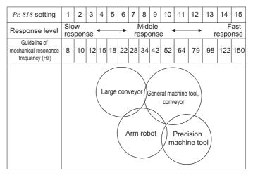
2) Each control gain is automatically set from the load inertia ratio estimated during acceleration/deceleration operation and the *Pr. 818 Easy gain tuning response level setting* value.
