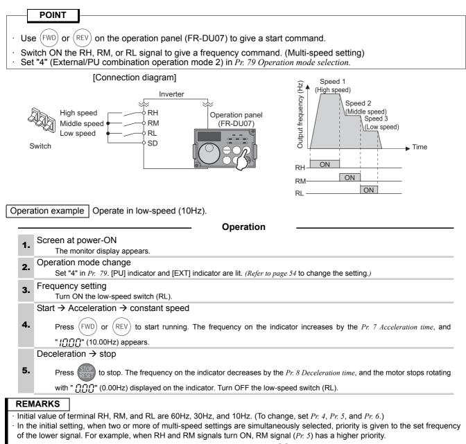
· Maximum of 15-speed operation can be performed. (Refer to Chapter 4 of 2) the Instruction Manual (Applied).)
