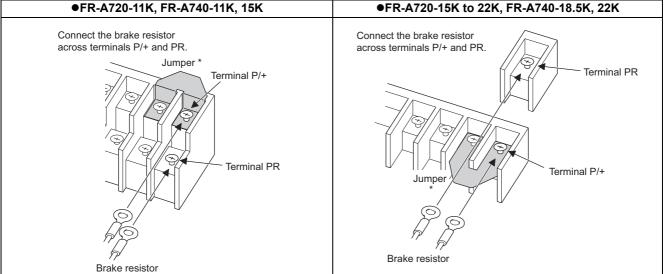
Do not remove the jumper across terminal P/+ and P1 except when connecting a DC reactor (FR-HEL).
