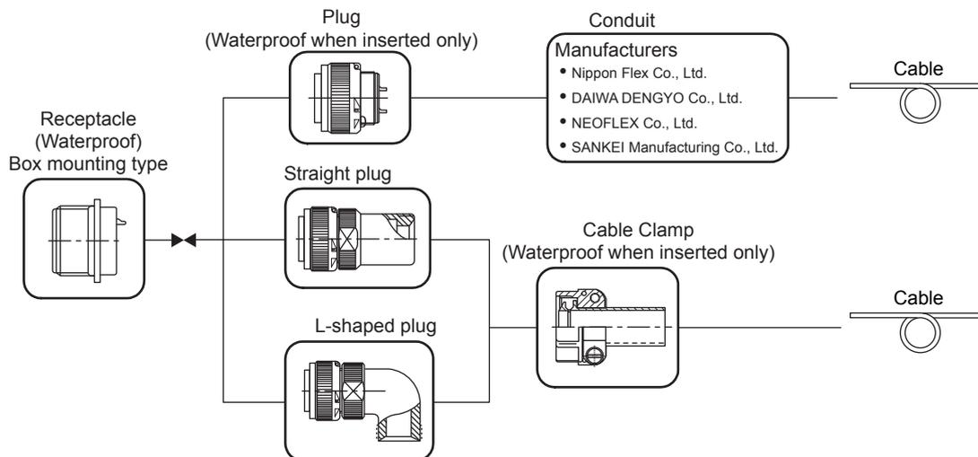
Note: Possible to connect with an MS connector
