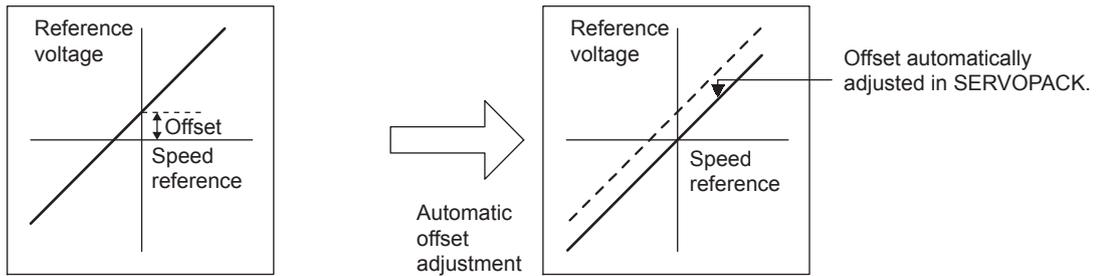
After completion of the automatic adjustment, the amount of offset is stored in the SERVOPACK. The amount of offset can be checked in the speed reference offset manual adjustment mode (Fn00A). Refer to 8.5.3 (2) *Manual Adjustment of the Speed Reference Offset*.
