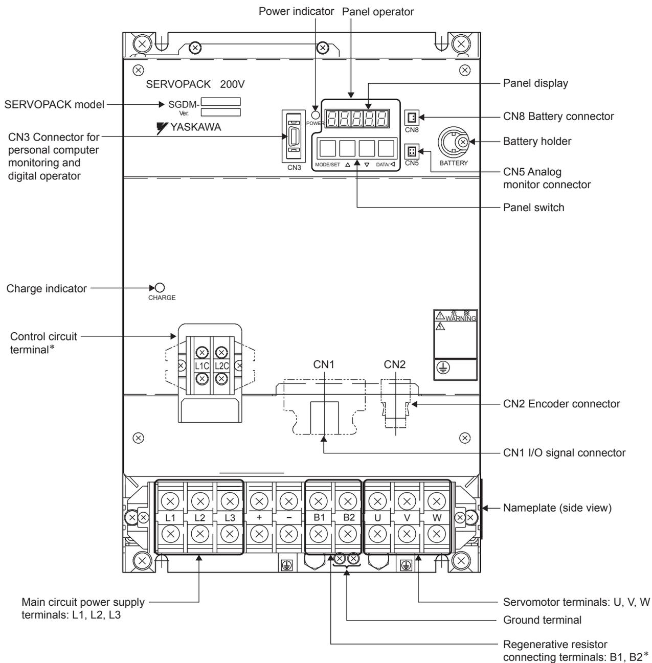
\* Control circuit terminal and regenerative resistor connecting terminals differ the position of the terminal block by the SERVOPACK model.
