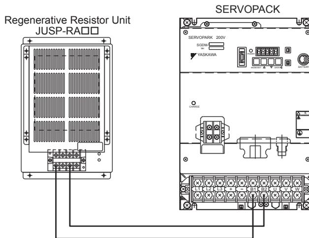
Note: Connect a regenerative resistor unit between B1 and B2 terminals. The regenerative resistor unit is provided by the customer.
