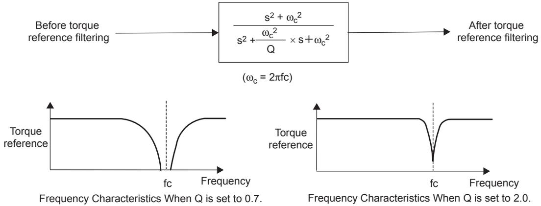
Note: The frequency characteristics shown above indicate that no response of the speed proportional gain can be obtained if the difference between the speed proportional gain and the vibration frequency is too small.
