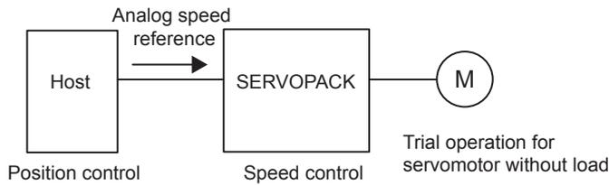
When the SERVOPACK conducts speed control and position control is conducted at the host controller, perform the operations below, following the operations in (2) *Operating Procedure in Speed Control Mode* ( $Pn000 = n.\square\square0\square$ ) on the previous page.
