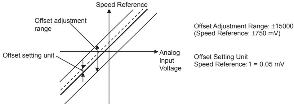
Adjust the speed reference offset manually in the following procedure.
