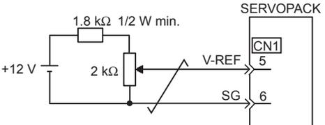
Connect V-REF and SG to the speed reference output terminals on the host controller when using a host controller, such as a programmable controller, for position control.
