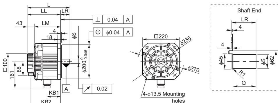
Note: For the specifications of the other shaft ends, refer to 3.20 Shaft End Specifications for SGMGH, SGMSH and SGMDH Servomotors.
