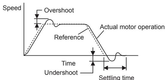
The mode switch function automatically switches the speed control mode from PI control mode to P control<sup>1</sup> mode based on a comparison between the servo's internal value and a user-set detection level.
