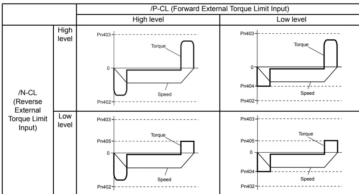
Note: In this example, the servomotor rotation direction is Pn000 = n.□□□0 (standard setting, CCW = forward).
