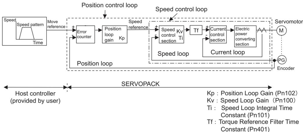
To adjust the servo gain manually, understand the configuration and characteristics of the SERVOPACK and adjust the servo gain parameters one by one. If one parameter is changed, it is almost always necessary to adjust the other parameters. It will also be necessary to make preparations such as setting up a measuring instrument to monitor the output waveform from the analog monitor.
