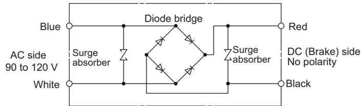
■ Noise Filter for Brake Power Supply
