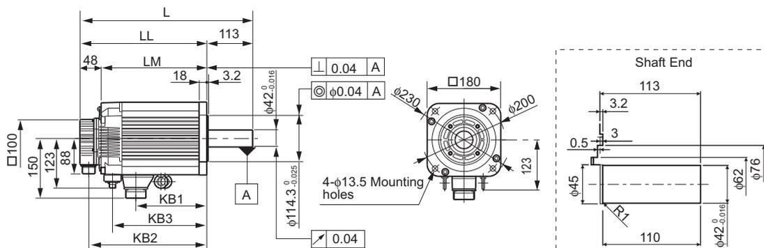
Note: For the specifications of the other shaft ends, refer to 3.20 Shaft End Specifications for SGMGH, SGMSH and SGMDH Servomotors.
