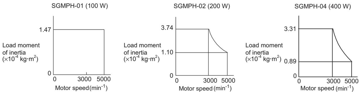
**(3) Allowable Load Moment of Inertia at the Motor Shaft**
