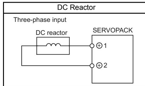
Note: 1. The SERVOPACK ⊕1 and ⊕2 terminals for the DC reactor are short-circuited before shipment.
