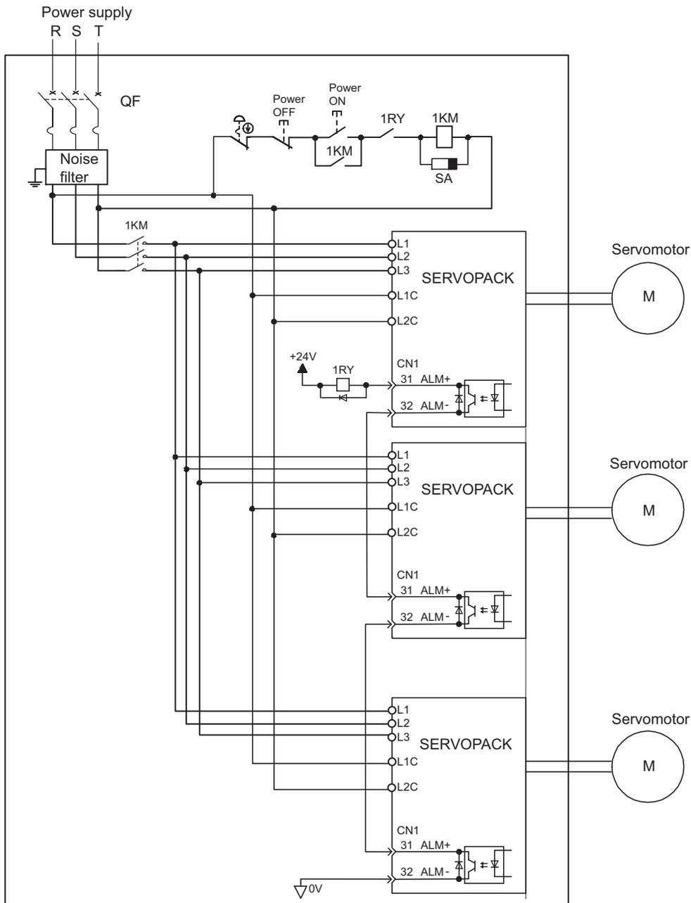
Note: Wire the system, so that the phase-S power supply will be the ground phase.
