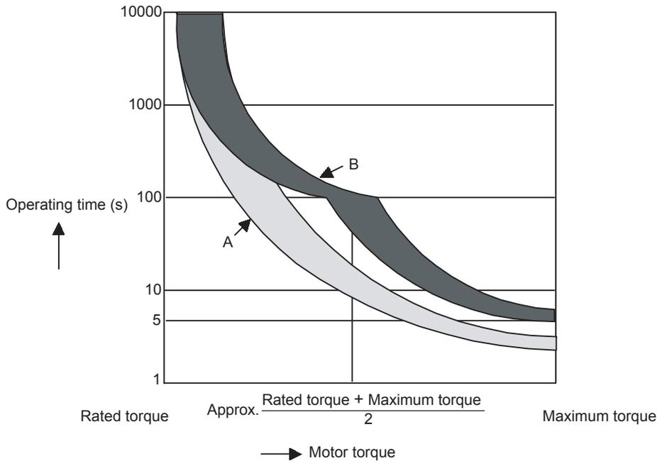
Note: The overload protection characteristics of A and B in the figure are applicable when the SERVOPACK is combined with one of the following servomotors.
