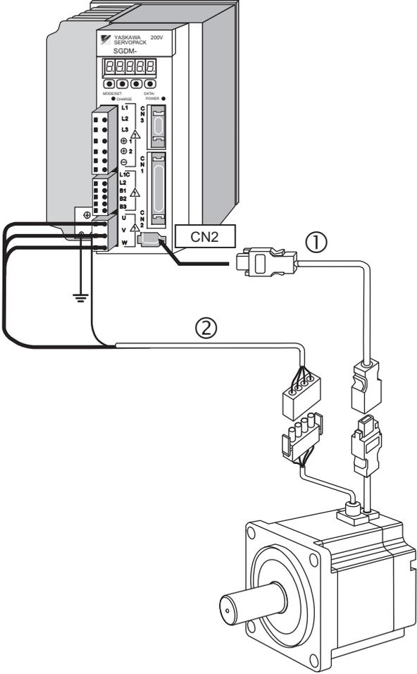
2.4.1 Cables for SGMAH and SGMPH Servomotors
