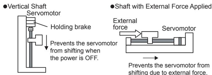
There is a delay in the braking operation. Set the following ON/OFF timing. The timing can be easily set using the brake interlock output signal.
