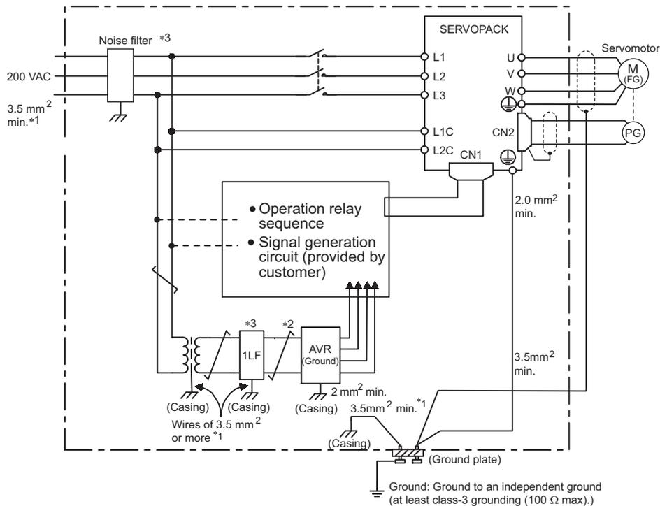
\*1 For ground wires connected to the casing, use a thick wire with a thickness of at least 3.5 mm<sup>2</sup> (preferably, plain stitch copper wire)
