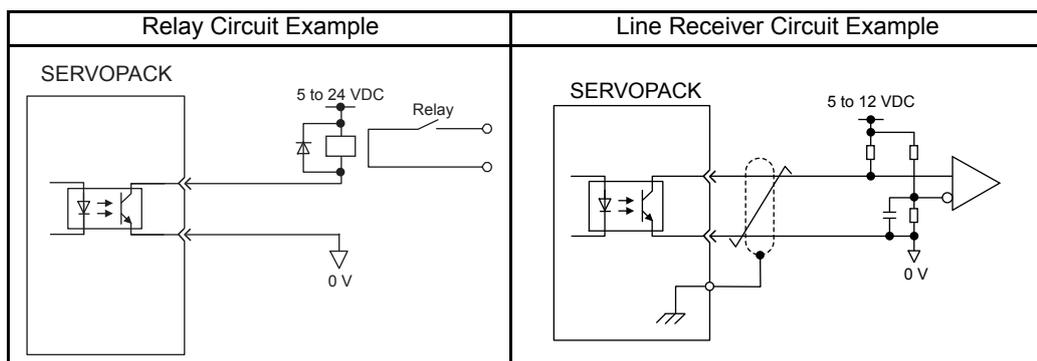
Note: The maximum allowable voltage and current capacities for photocoupler output circuits are as follows:
