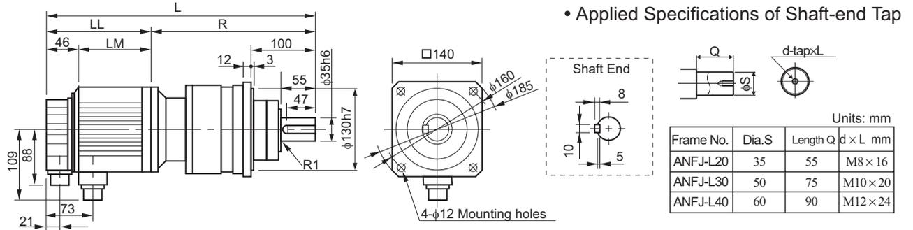
• Detailed Dimensions of Gears
