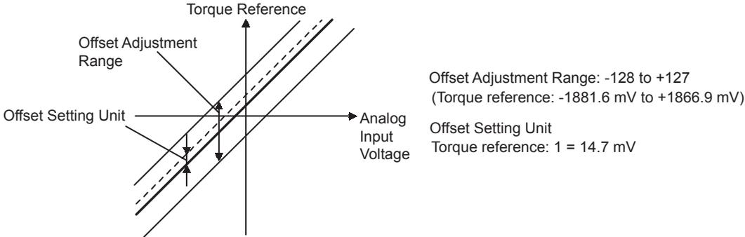
Use the following procedure to manually adjust the torque reference offset.
