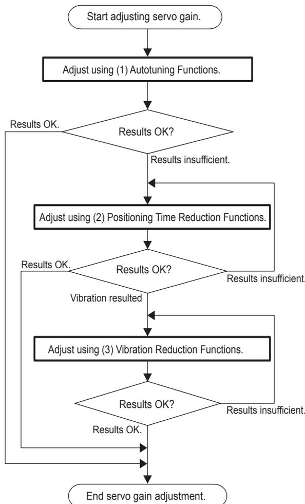
If the desired responsiveness cannot be achieved adjusting according to the servo gain adjustment methods, consider the following possible causes.
