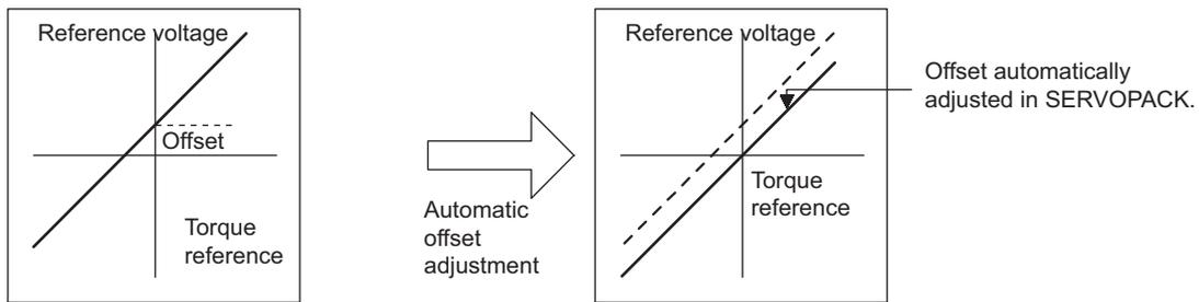
After completion of the automatic adjustment, the amount of offset is stored in the SERVOPACK. The amount of offset can be checked in the manual adjustment of torque reference offset (Fn00B).
