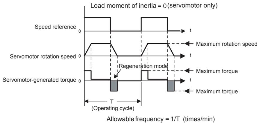
Fig 12.1 Operating Conditions for Allowable Regenerative Frequency Calculation
