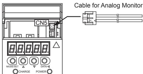
Note: Specify the cable type either JZSP-CA01 or DE9404559 when ordering the cable for analog monitor.
