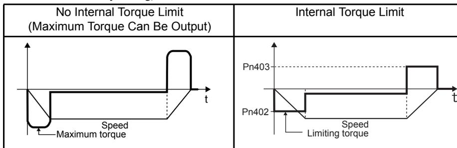
Too small a torque limit setting will result in insufficient torque during acceleration and deceleration.
