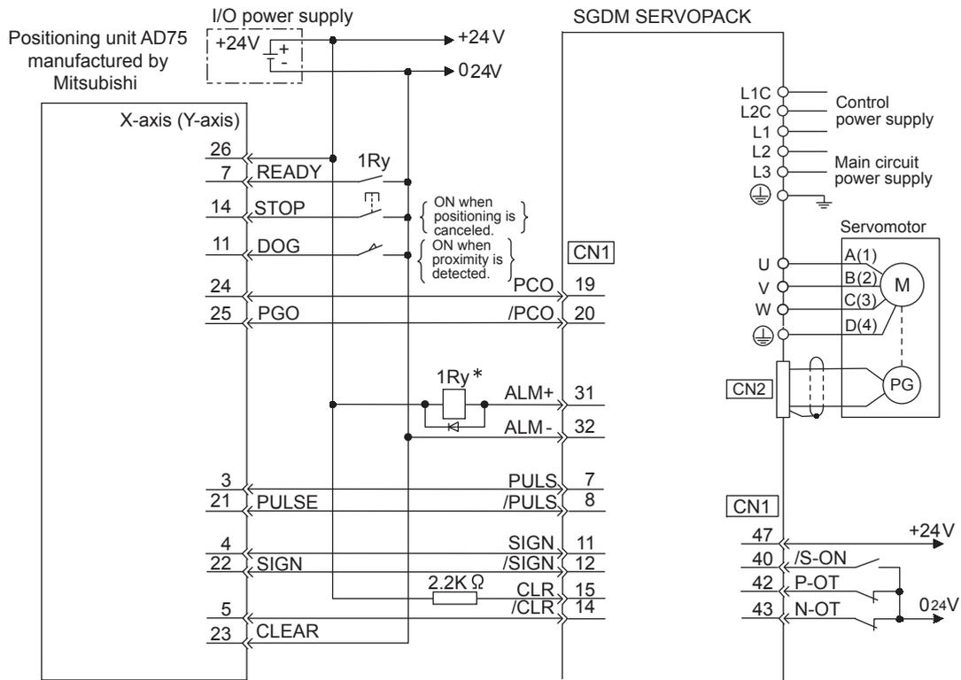
\* The ALM signal is output for about two seconds when the power is turned ON. Take this into consideration when designing the power ON sequence. The ALM signal actuates the alarm detection relay 1Ry to stop the main circuit power supply to the SERVOPACK.
