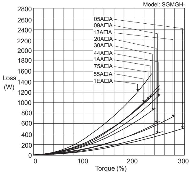
SGMGH Servomotors (1000 min<sup>-1</sup>)
