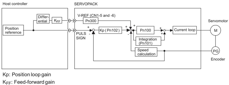
Speed feed-forward value is set using the parameter Pn300.
