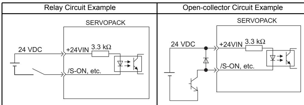
Note: The 24 VDC external power supply capacity must be 50 mA minimum.
